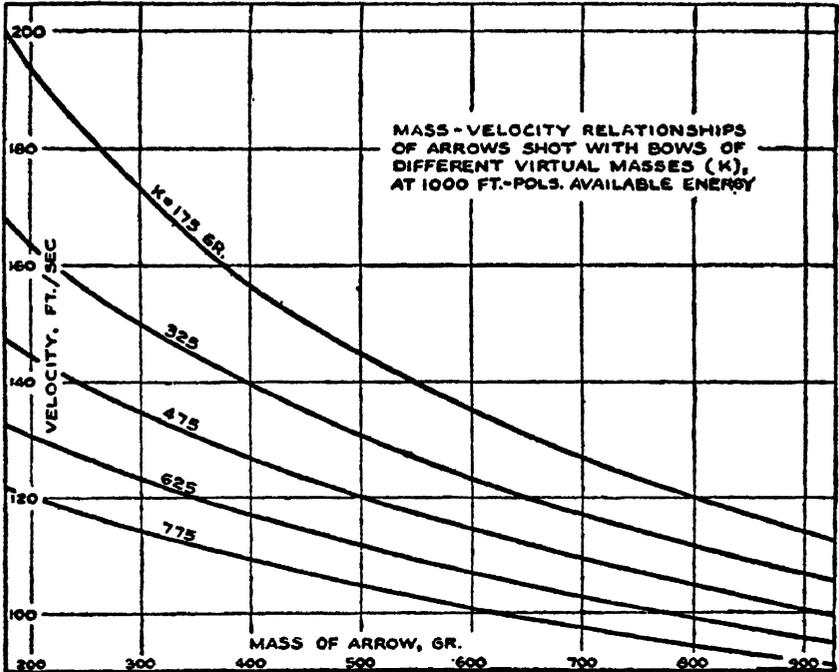
FIGURE 10.—A set of curves relating mass of an arrow to its velocity when shot from bows of different virtual mass but the same available energy.
