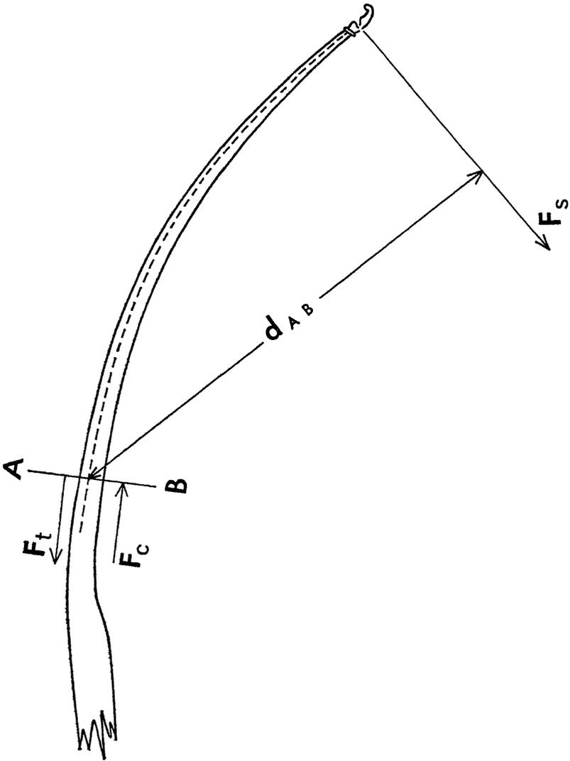
FIGURE 4.—Schematic side view of a bent limb. The dotted line indicates location of the neutral layer.
