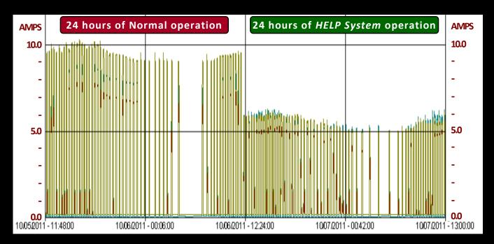
Independent testing of energy consumption on a 7.5-ton Trane air conditioner
