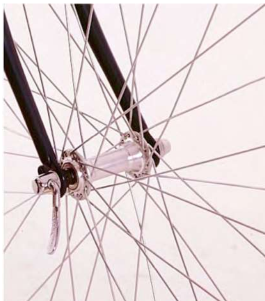
Figure 6 Quick Release Incorrect Position—Example 1
