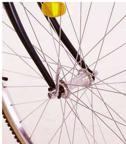
Figure 7 Quick Release Incorrect Position—Example 2
