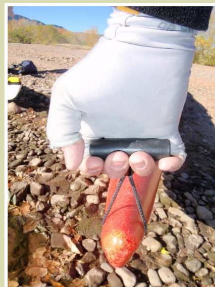
Figure 2: The plastic barrel below the toggle caused blood blisters
