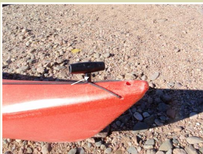
Figure 1: The original stern toggle configuration with an arrow pointing to the problematic barrel
