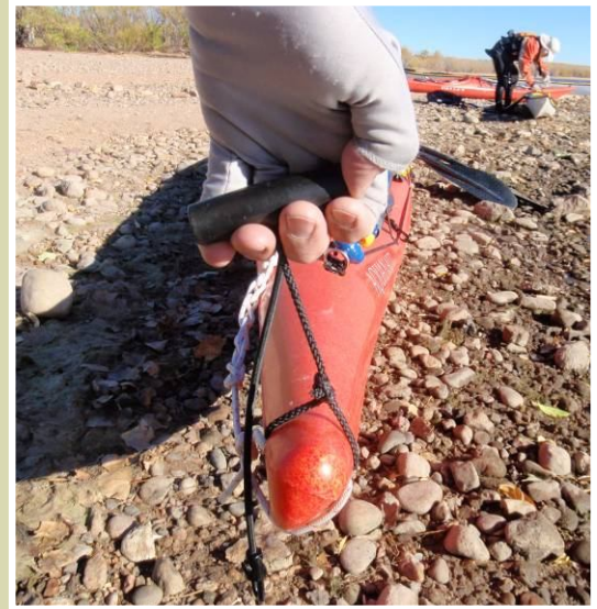
Figure 4: There is no barrel to pinch and the kayak is free to move as nature dictates without snapping a wrist
