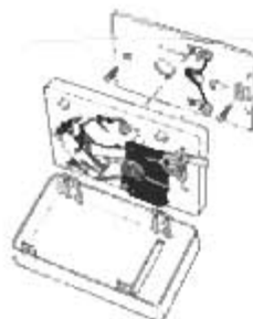
Fig. 1 Mounting and wiring with Sub Base (T80-300 and T80-400 only)
