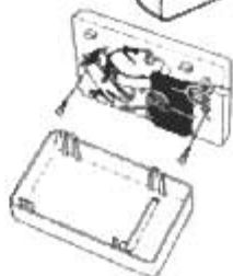
Fig. 2 Mounting and wiring without Sub Base.
