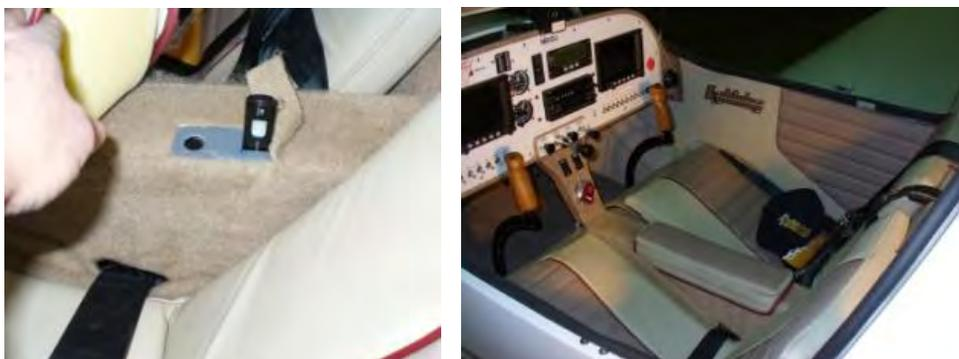
The second tip is just one of those little helpful tips, not a real biggie. My plane is equipped with boarding steps and I have noticed how easily the paint on the steps scuff from normal use. I found heavy duty adhesive coated shrink tubing at Fastenal (see picture for shrink tubing information). I cut two pieces 4-1/4 inches long and slid them over the boarding steps and used a heat gun to shrink and bond them in
