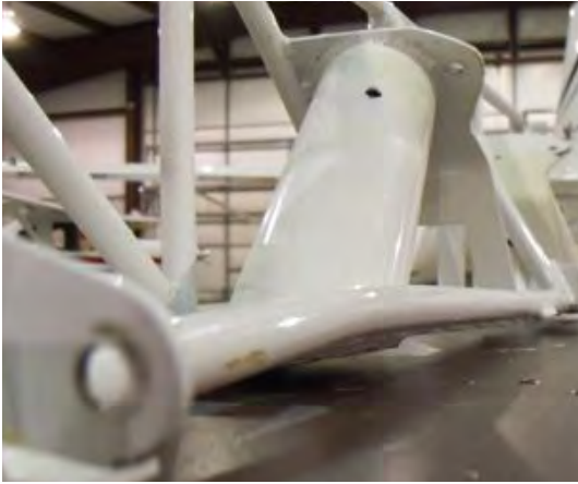
Figure 1: deformation of rear 1/2" tube box V1 socket plate V1
