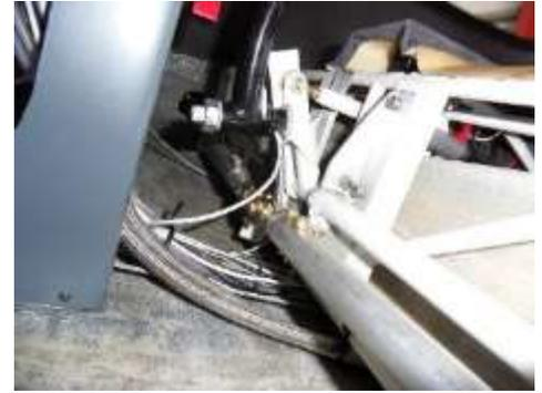
The central stick made two throttles a necessity. I had a "tactical throttle" on the left cabin wall in my first Lightning and I could use the parts in the new one. The copilot's throttle is the usual one, only mounted on the right panel box.
