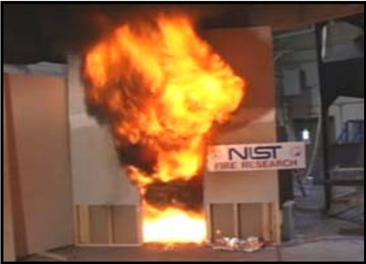
Figure 3 – Flashover and subsequent Backdraft
