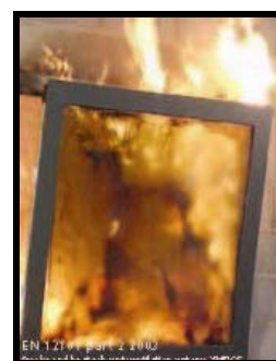
Figure 7 – EN12101.2 (BS 9999) fire test
