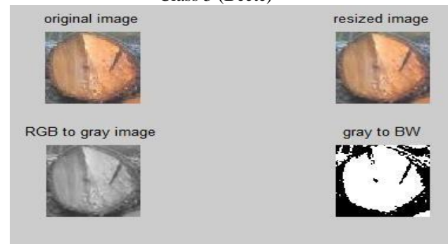
Fig.3: conversion of gray and binary image of beete wood log
