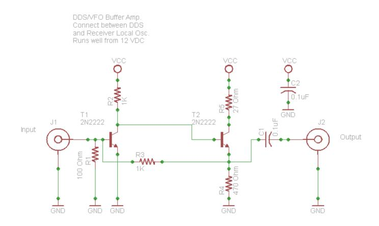
A 2N2222 transistor is specified; however any general purpose NPN transistor will suffice – may be built Manhattan style.
