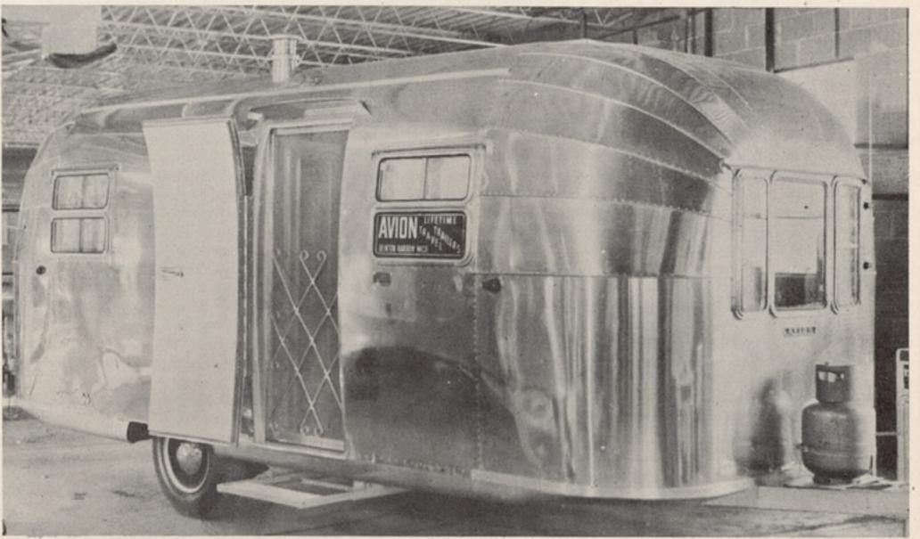
Avion Coach Corporation, Benton Harbor, Mich. introduces new 20 foot Rambler model travel trailer. Trailer's inside width at floor measures 7 feet and has an approximate overall weight of 2300 pounds. Two models are offered with choice of dinette or sofa converting to double bed.
