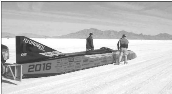
At the Bonneville Salt flats in October the Ohio State Buckeye Bullet 2 recorded the fastest ever speed for a hydrogen fueled and fuel cell powered vehicle at around 224 mph, and has set the official FIA world record for Group XIV-class 3 (fuel cell engine, unlimited weight) at around 130 mph. (Subject to FIA (or ASN) recognition).
