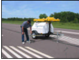
1. Level as necessary using 3 leveling jacks.
