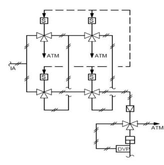
SOLENOID VALVE WITH 2003 VOTING, ONLINE COIL CHANGE-OVER FACILITY & PARTIAL STROKE TESTING
