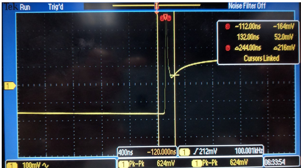
Figure 18. Measure from the start of the square-wave to the portion just before the exponential charging.
