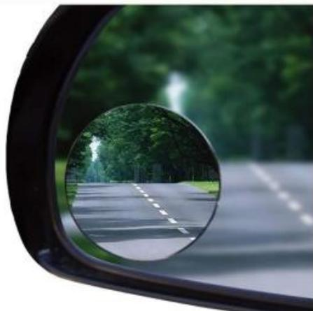
Here's my little Tech Tip: Add a small "bubble mirror" to the face of that flat mirror, using a couple of strips of two-sided tape. Hunt around for a bubble mirror that closely matches the diameter of your flat mirror. Look for them in auto parts stores, general merchandise stores, truck stops.
