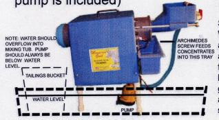
SUGGESTED WATER RECIRCULATING SYSTEM When using the Mountain Goat Trommel away from a running water source, we suggest you purchase a concrete mixing tub (the large size) and a bucket from your local Home Depot or Lowes. The talilings bucket must be emptied before overflowing to keep gravel out of the water supply. You should also slip a sock over the pump to help keep the the spray system from clogging up.
