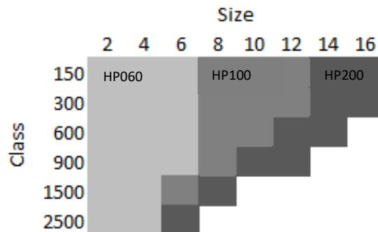
\*Size based on standard valve flange size
