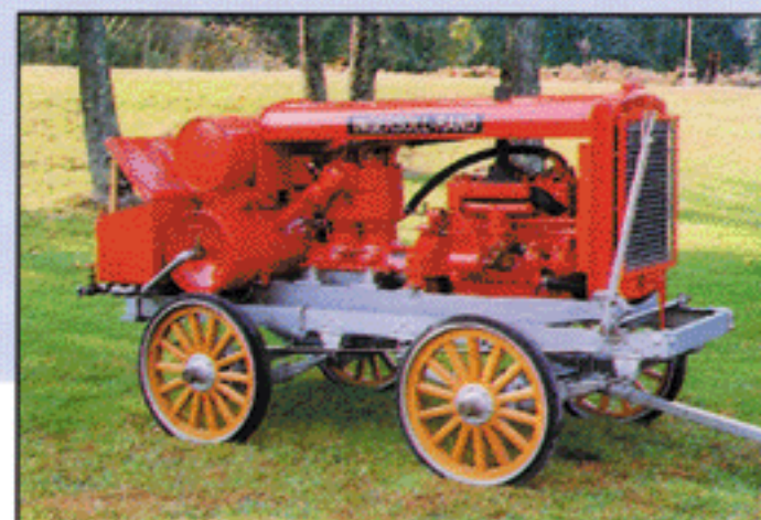
Restored 1930's Vintage Portable Air Compressor with Dollinger Protectomotor filter
