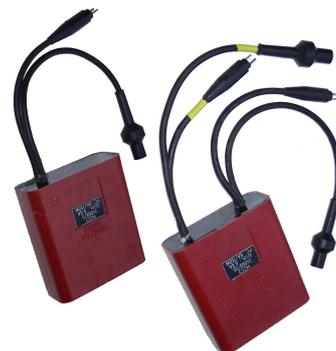
The series lighting cable is used as a signal carrier. The only installation activity required is to plug the Lamp Control/Monitoring Units (MCCs) into the series circuit between the isolation transformer and the light (or device) to be controlled or monitored. No other elements like filters or by-passes are required.
