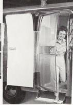
NEW COMBINATION DOOR and SCREEN - Full-size hinged screen door swings open. Keeps insects outside. Latches easily to main door when desired. Provides more interior living space.
