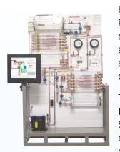
Hampden H-RST-2-CDL-DEMO Refrigeration System Trainer was designed to provide students with an actual working model of a refrigeration system, complete in every
