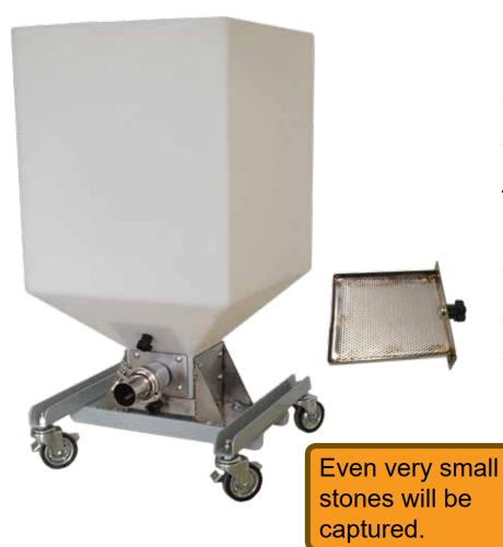
Remove stones and other dense particles. Run at rates up to 1200 pounds per hour. Stainless steel separator 3 Cu. Ft. PE hopper Adjustable flow Easy clean design. Cut to match Cooler Steel frame, 4 locking casters Stone collection drawer
