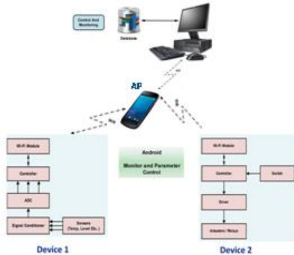
Fig 2: System block diagram of intelligent d2d communication with Wi-Fi using IoT
