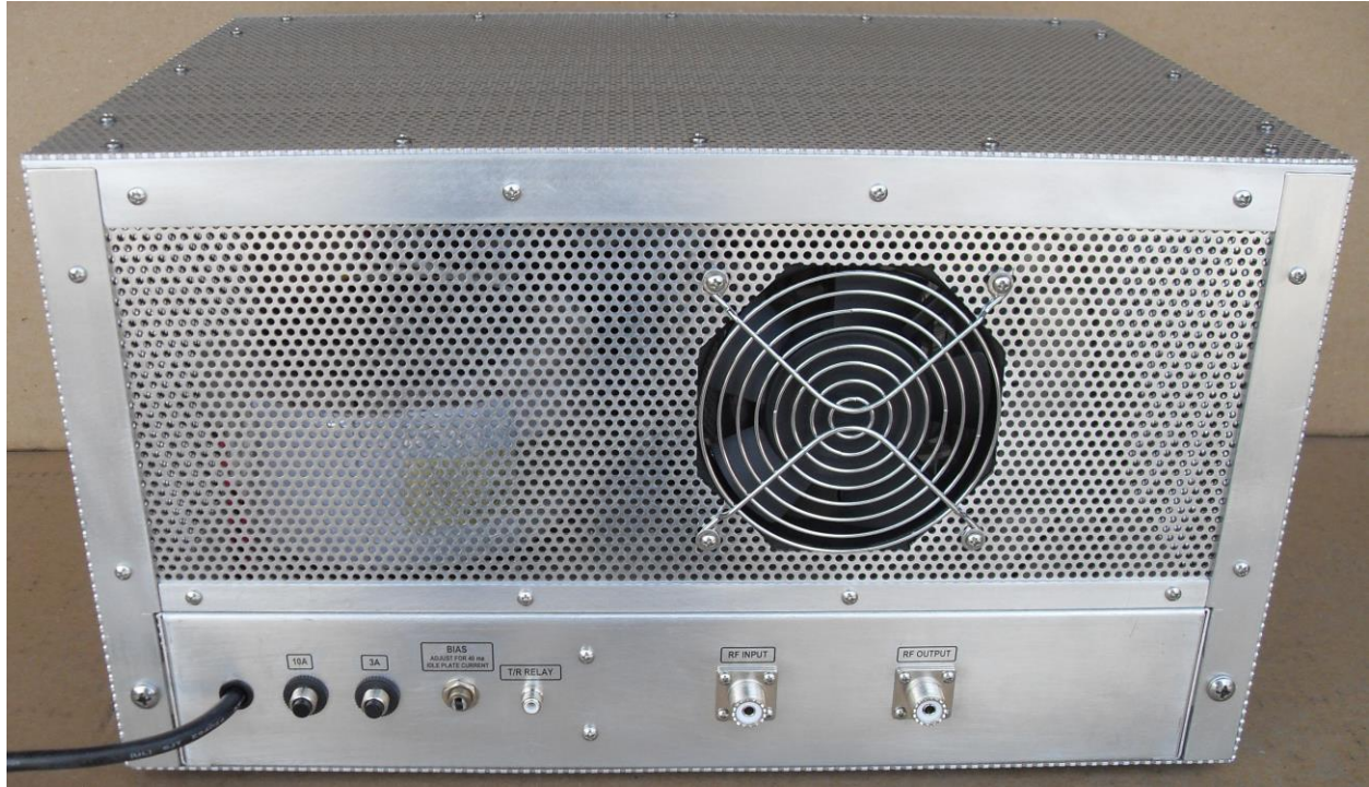
Figure 4: Rear View with Cabinet Installed
