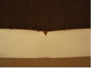
Knit line and V-groove close-up (after conditioning)
