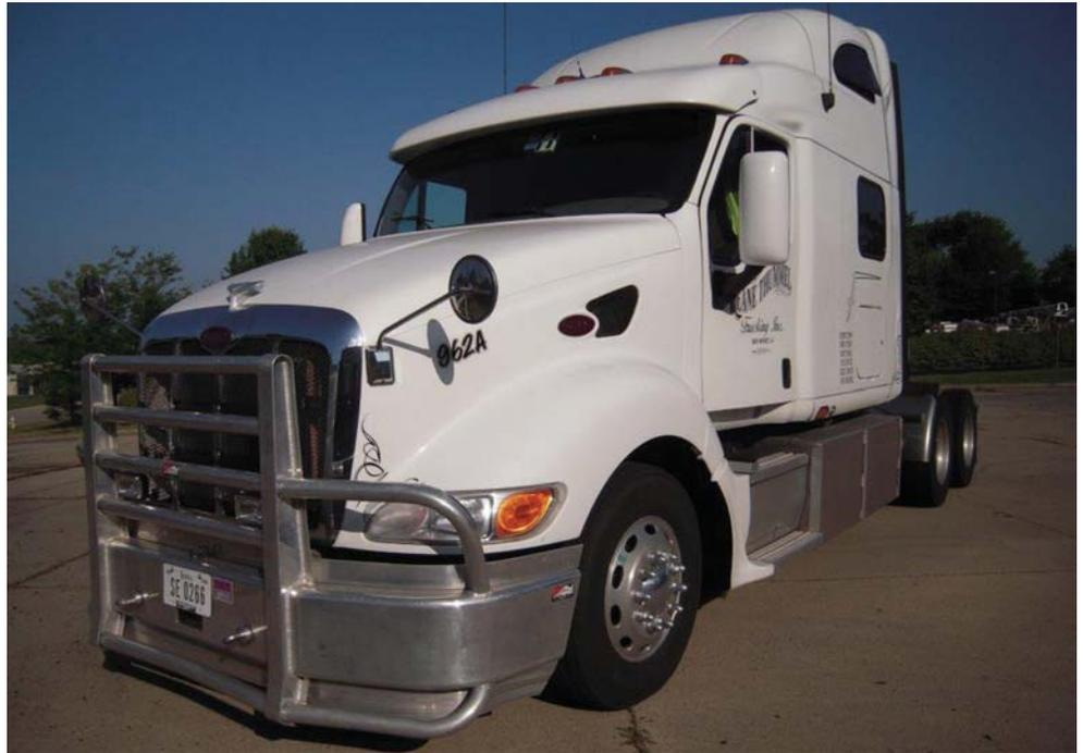
**The converted truck with battery boxes mounted on the outside, immediately behind the steps to the cab**
