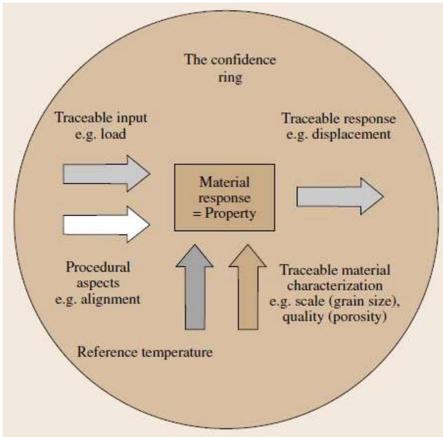
Confidence ring for material property combined measurement and testing – note that separate traceability requirements apply to applied stimulus (load), response (displacement), and material characterization (grain size, porosity)
