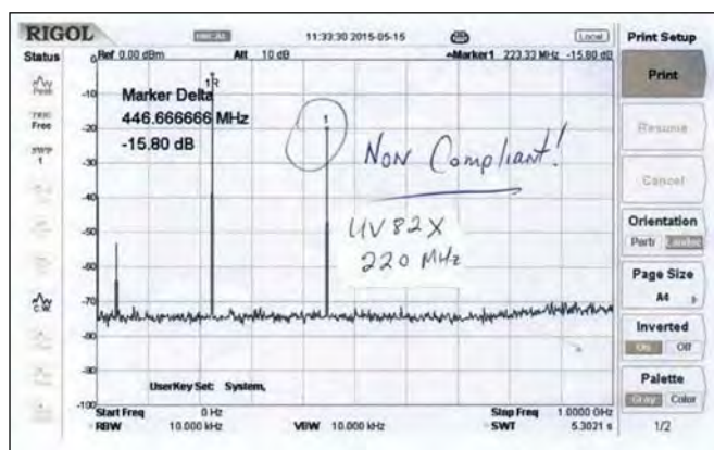
Figure 4 — This Baofeng UV82X does not comply with the FCC spectral requirements of Part 97.307e. The second harmonic of the fundamental signal is only 15.8 dB below the strength of the desired output signal.
