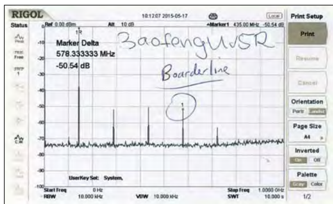
Figure 3 — Here is the spectral output for another Baofeng UV5R, which is borderline compliant with the FCC spectral requirements. Note that there are several signals that are approximately 50 dB below the strength of the fundamental output.
