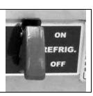
5) When the product has frozen to the desired stiffness, immediately turn OFF the refrigeration switch, and begin to discharge the product.
