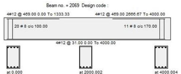
Figure 3. Reinforcement details for beam
