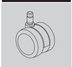
2<sup>1</sup>/<sub>2</sub>-inch-diameter doublewheel caster; black nylon wheels and yoke; soft polyurethane tread; internal brake; for use on hard floors
