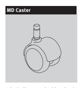
2-inch-diameter double-wheel caster; black nylon wheels with integral chrome hood; soft polyurethane tread; for use on hard floors or carpet Applicable on:
