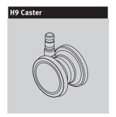
2<sup>1</sup>/<sub>2</sub>-inch-diameter doublewheel caster; clear polycarbonate wheels; nylon yoke; soft polyurethane tread; for use on carpet only
