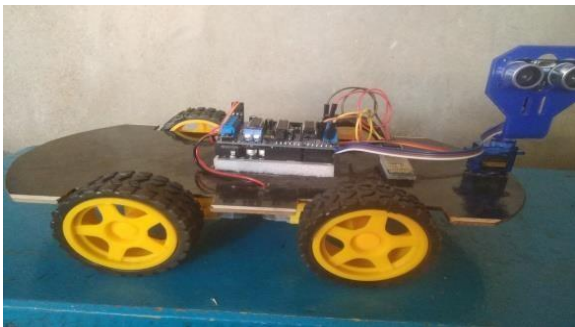
Fig. 4. Sample for hardware implementation of voice control robotic vehicle
