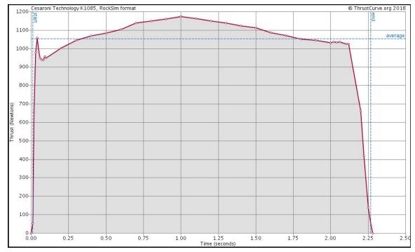
3.3.2.4 Simulated Motor Thrust Curve
