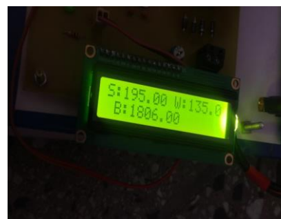
Fig. 6: Monitoring using 16x2 LCD Display
