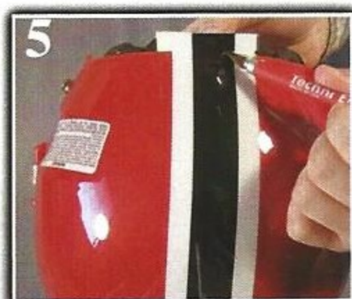
5) When multi-tape is completely applied, there may be excess vinyl. Trim excess vinyl from back of helmet so the tape edge is flush with back edge of helmet.
