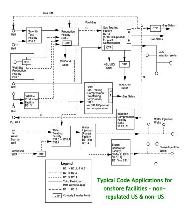
used, then ASME B31.4 (liquids) or ASME B31.8 (gas or liquid and gas) may be more appropriate and cost effective.
