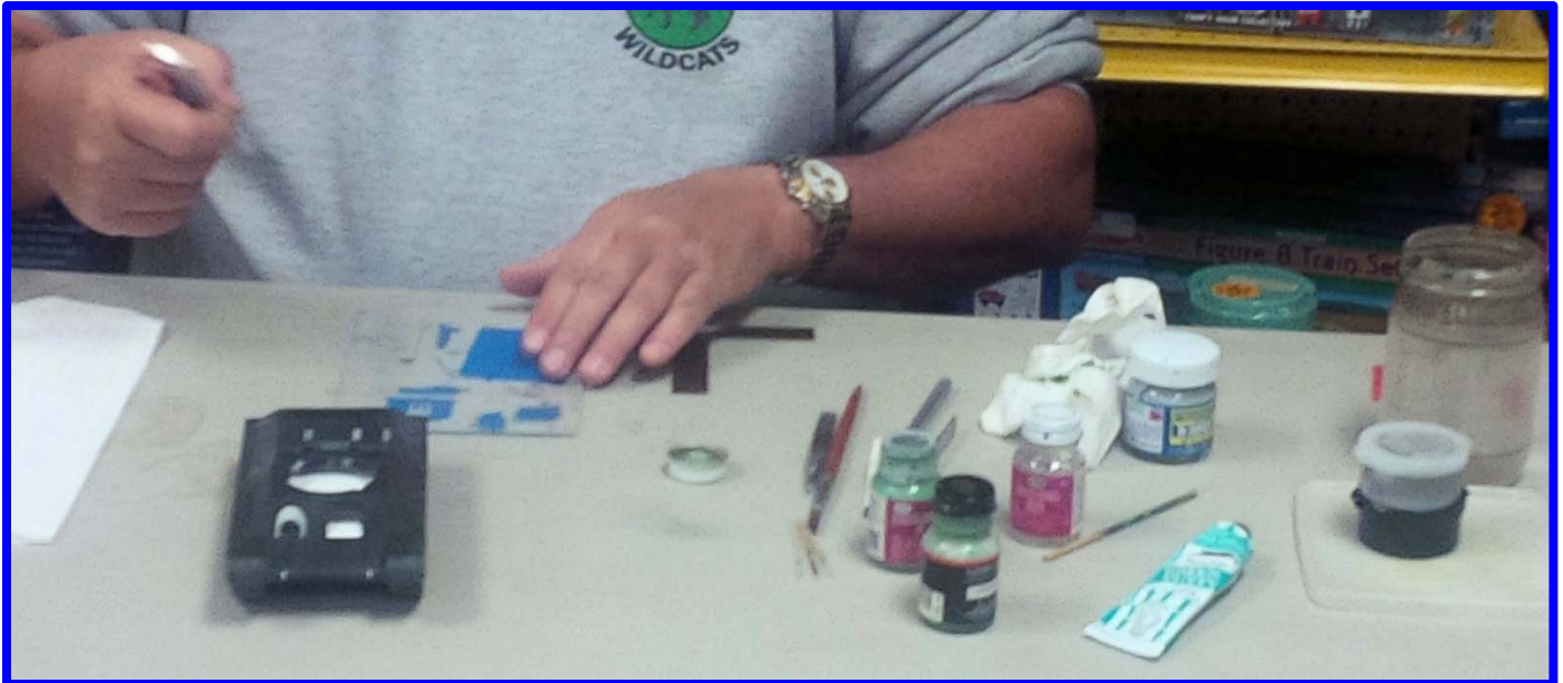
Mike cuts thin strips of Painters Tape on a piece of glass using a sharp blade & straight edge
