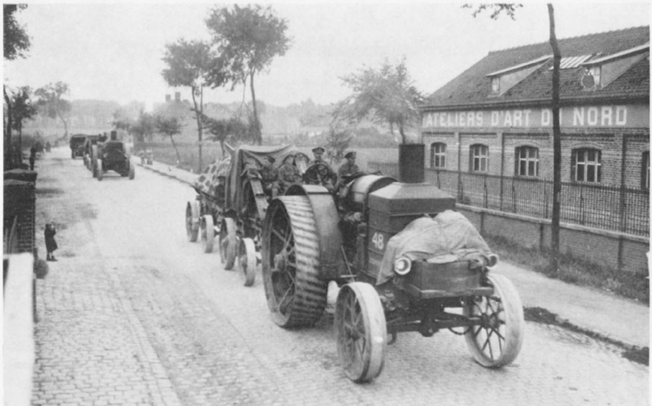
Progenitors of the Tank 1: the Foster-Daimler petrol (gasoline) tractor (shown in use by the Royal Marines Artillery), the engine of which was to be used for the projected "big wheel" machine and which was subsequently used to power all tanks Mk. I-IV. (Chamberlain Collection)
