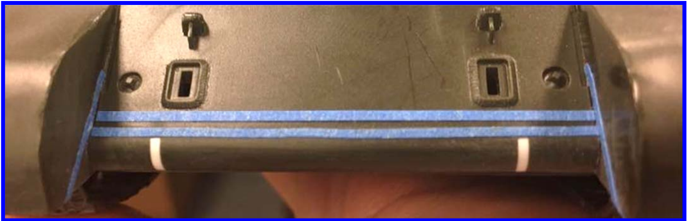
Thin strips of Painters Tape placed in parallel lines to define the Weld Bead
