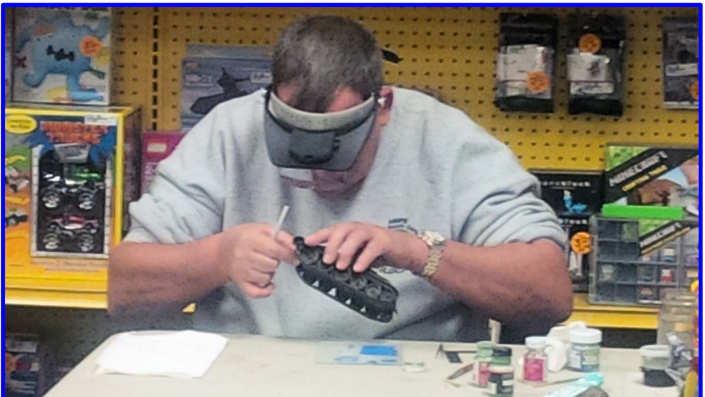
Mike then installs the tape strips on the hull where he wants to make a Weld Seam
