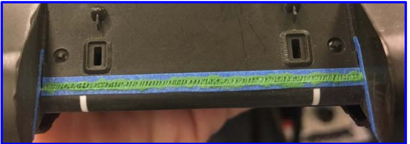
While the Putty is still soft, the Tool Tip is repeatedly pressed into the Putty Surface
