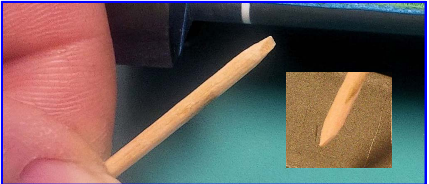
Mike created a Sculpting Tool by cutting a Chisel Point on one End of a Tooth Pick
