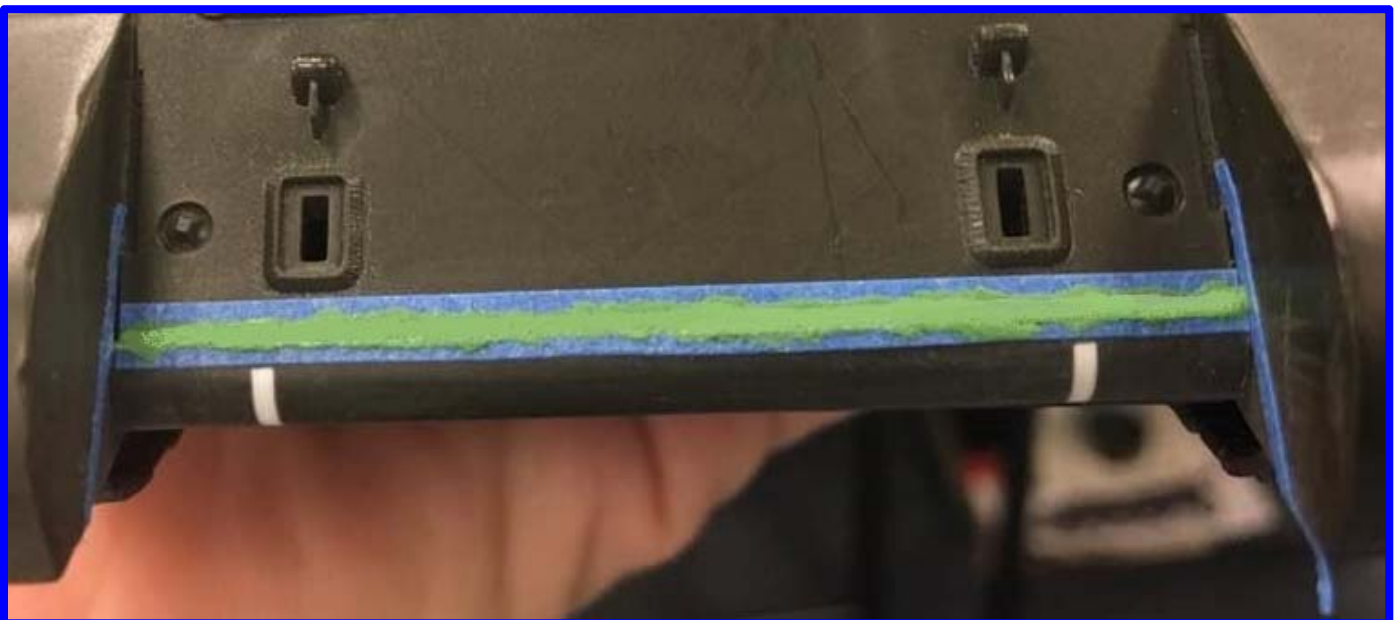
Thinned Putty is "Painted" over the Tape Strips and Gap
