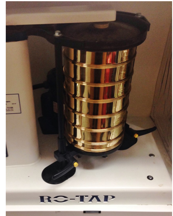
Ro-Tap machine containing 7 sieves and a bottom pan
