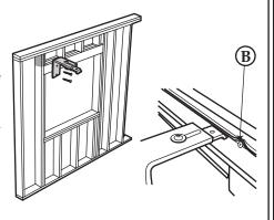
3. Adjust projection of bracket clip by loosening the screw nut (A). Adjust bracket projection as needed. Retighten the screw nut to hold the clip in desired position.
