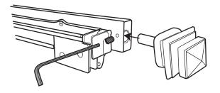
5. Clip traversing track onto the brackets on the wall; make sure track is securely in brackets.
