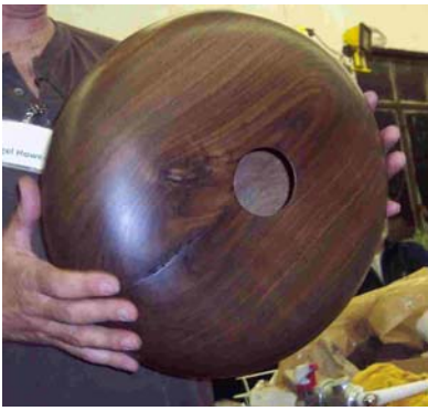
Nigel a Black Walnut hollow form turned with homemade tools finished with Tung oil and mineral spirits and an Oak burl bowl (One of his smallest ever turnings?)
