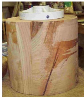
Ken is making a mold for a glassblower client to insert molten glass into and then inflate into the inner shape as shown by his drawing
