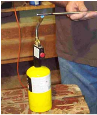
Bending the end by heating it with MAP gas
