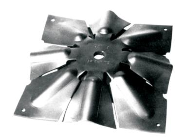
The eight blade, one-piece top plate, deeply embossed for additional strength, expands upon impact into undisturbed earth to form a pyramid shaped square. The 8-way anchor retains its shape under extremely heavy loads due to the support of the eight blades by the base plate.
