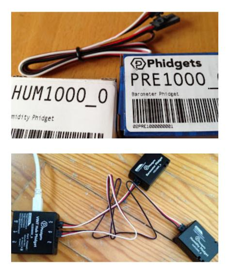
For now we added support for the Phidgets VINT HUM1000 and PRE1000 modules which allow to measure relative humidity and absolute air pressure which is converted to barometric pressure taking the given elevation of the roasting location into account. You can configure ambient sensors in the Device Assignment dialog (menu Config >> Device, last tab Ambient). We plan to add support for further "weather stations" in the future.
