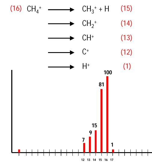
Single Ionization occurs when electron impact (EI) causes CH<sub>4</sub> to lose an electron, becoming CH<sub>4</sub><sup>+</sup>
