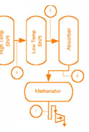
(4) High Temperature and (5) Low Temperature shifts remove the CO to increase the production of  $H_2$ .
