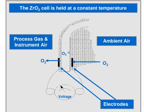
• A voltage potential corresponding to the partial pressure is generated as the oxygen moves from one electrode to the other
