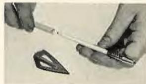
The lightweight, precisely-wound bobbin is attached to the broadhead insert and contains 3,000 feet of trail.
