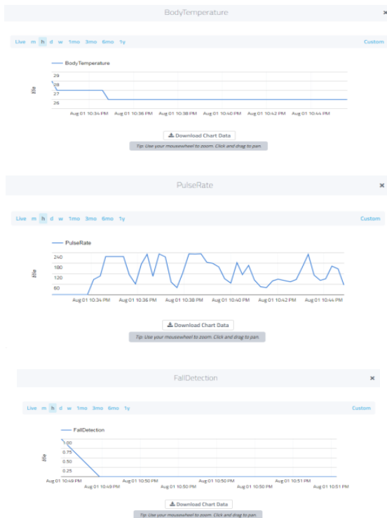
Fig.3: Temperature, Pulse Rate, Fall Detection readings as displayed in Cayenne Cloud
