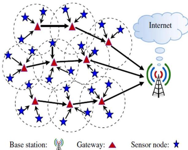
**Fig. 1: A Wireless sensor network model**
