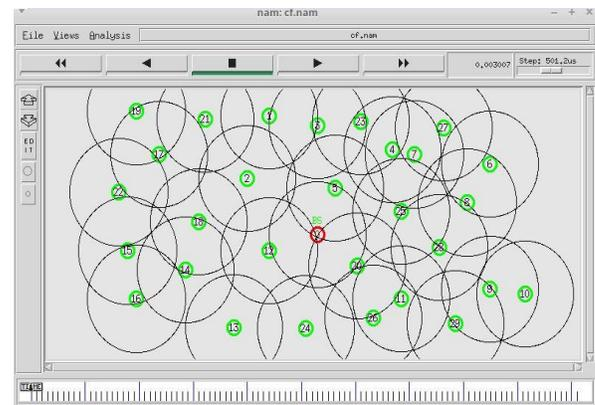
**Fig. 4: Nodes exchanging Hello packets**
