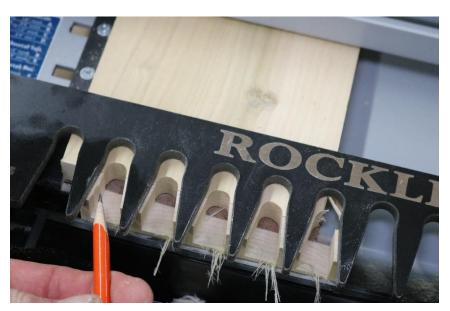
When cutting through sockets, the first pass should be very light, much like the scoring cut on half-blind dovetails, to minimize chip out.
