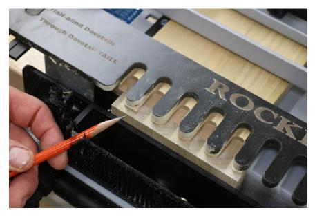
Before removing the boards from the jig, make certain there aren't any spots you missed with the router. It's nearly impossible to get the parts back in the jig in exactly the same position.
