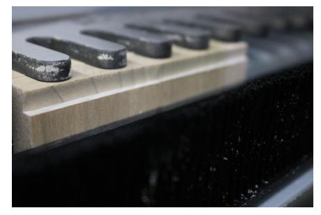
Start with a scoring cut on the face of the vertical piece.
