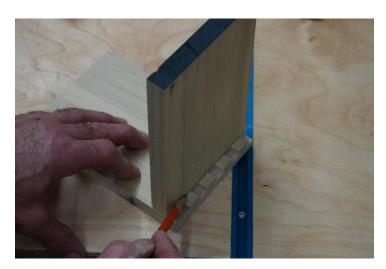
Cut and assemble the joint. Trace the face of the tail board onto the sockets. This tells you where to cut the rabbet.
