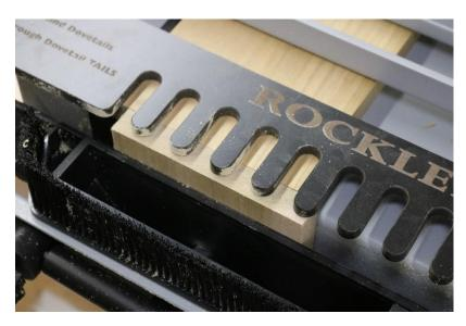
Be very careful loading the material in the jig. Make certain the horizontal and vertical pieces meet, and that the end grain of the vertical piece is even with the top face of the horizontal. Double check that the edges of the pieces are against the stop.
