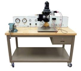
Provides students with hands-on training for valves, positioners, and actuators found in industry today. Students learn the operation and servicing of globe, ball, and butterfly valves, and both pneumatic and electro-pneumatic positioners and actuators. This trainer is complete with all of the necessary pneumatic and electronic power supplies, connectors, gauges, and regulators necessary to perform experiments utilizing the various valve assemblies.
