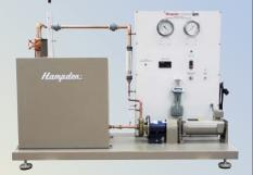
44 gallons (167 liters) of water. Also mounted on the base is a Centrifugal Pump with gauges (mounted on panel) to indicate its suction (input) pressure (vacuum) and its discharge (output) pressure. The demonstrator provides two methods of determining flow rate which can be manually adjusted with a Throttle Control Valve.
